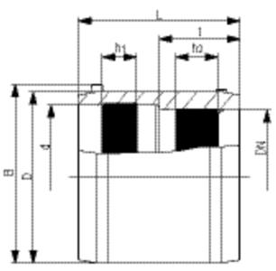
PE 100 SDR 17 Maximum permissible working pressure 10 bar (water) / 5 bar (gas)
