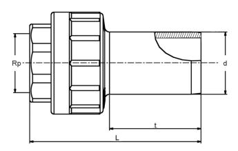
PE 100 SDR 11  $$\operatorname{Maximum}$  permissible working pressure 16 bar (water) / 5 bar (gas)
