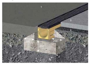
Road concrete and / or concrete sheets or paving bed Cast asphalt
