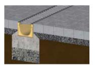
6. Install paving. The layer should end 2 to 5 mm higher than the cover grating.
