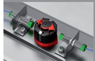
Inductive switches indicating open and closed position
