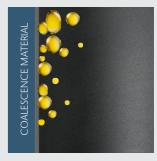
The adhesion of the oil film is exceeded. A large drop of oil begins to separate, floats upward and can therefore be separated.
