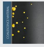
Oil droplets spread over the coalescence material, and additional oil droplets are adsorbed and the oil film continues to grow.
