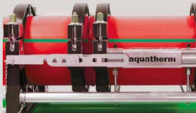
Join the pipes, cool down under pressure
