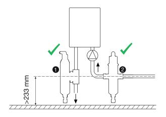
A dirty, problematic system would benefit from installing the combined unit in the return pipe, as close to the boiler as practically possible, or after the last tee connection in the return line. The small waterways in boilers do need consideration depending on system circumstances.
