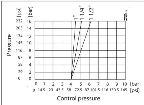
Figure 5: Control head  $\varnothing 110$  mm / 4 1/2 in
