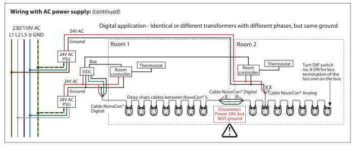
Wires that ends in an "X" must be properly terminated.
