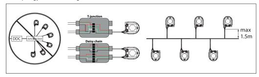
If the supply voltage to the first device in the daisy chain is lower than 24V AC/DC, or long thin cables other than NovoCon® cables are used, then the quantity of devices in the daisy chain may have to be reduced.
