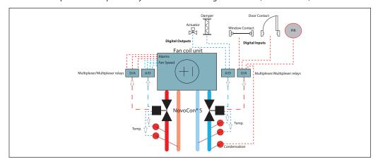
Application principle: Central Plant Changeover – 2 pipe system
