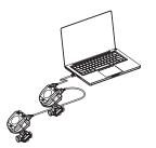
When using modbus function 21 (0x15) to update the firmvare in NovoCon® S it is nessecasy to perform the upload in smaller sections due to modbus limitations in file size, please see the modbus standard for more details.
