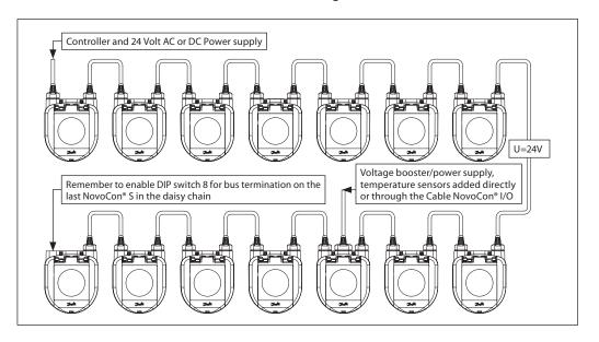
When all devices on the sub-network are NovoCon® S, refer to the examples below for guidance.
