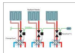
Separate maximum flow pre-setting for heating and for cooling
