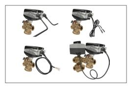
NovoCon® S is a high accuracy multi-functional field bus actuator, specifically designed for use in combination with the Pressure Independent Control Valve type AB-QM in sizes from DN 10-32. The flow is modulated by the AB-QM pressure independent control valve to avoid overflow and reduced boiler and/or chiller efficiency.
