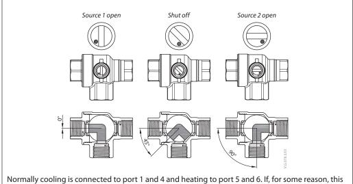
Normally cooling is connected to port 1 and 4 and heating to port 5 and 6. If, for some reason, this is not the case, then Inverted CO6 mode (MSV:9/32810) must be used instead.
