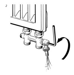
When the drain tap has been mounted (1), open by turning the Allen key (2).
