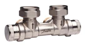
The valve has an integrated differential pressure control, that ensures constant pressure over the radiator valve. The flow adjustment presetting is done on the radiator valve. Based on constant pressure.
