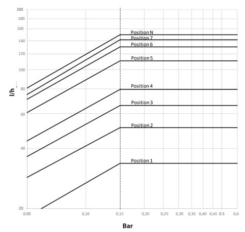
(Capacities comply to all radiators inside a -+ 10% span depending on the radiator type and size.)
