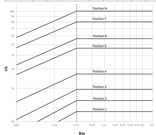
(Capacities comply to all radiators inside a -+ 10% span depending on the radiator type and size.)
