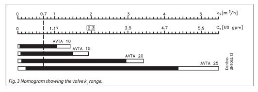
$K_{\rm v}$  values are always given for water flow in [m³/h] with a pressure drop  $\Delta p$  of 1 bar. The valve should be selected so that the necessary  $k_{\rm v}$  value lies in the middle of the regulation range.
