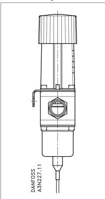
The valves can be installed in any position. An arrow on the valve body indicates the direction of flow.
