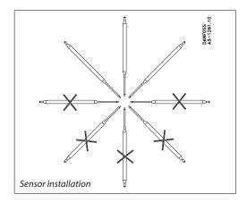
The charge is a mix of liquid and gas. Due to the mixture of liquid and gas the sensor must be installed in an area or environment that is warmer than the valve.
