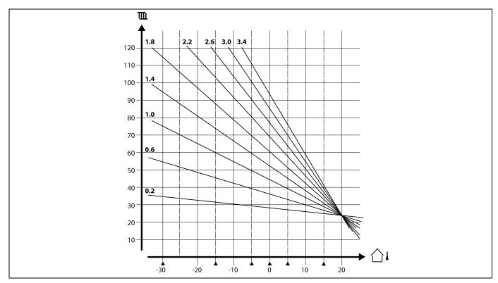
The small arrows (**A**) indicate 6 different outdoor temperature values at which you can change the heat curve.
