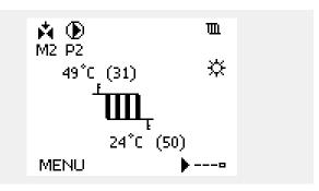
Display example with heat exchanger:
