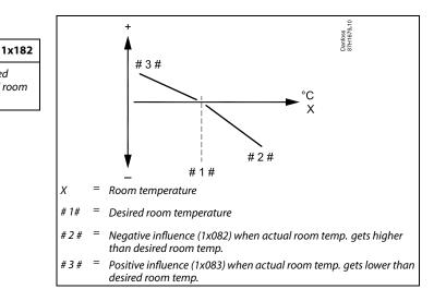
The 'Infl. - max.' and 'Infl. - min.' determine how much the room temperature should influence the desired flow temperature.
