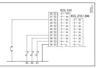
Example: Connection of an override relay
