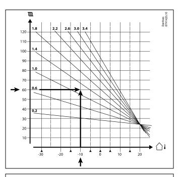
Choose the desired flow temperature (vertical axis) for your heating system at the expected lowest outdoor temperature (horizontal axis) for your area. Pick the heat curve closest to the common point of these two values.
