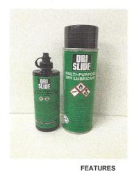
**Appearance** Black liquid Odor Mild petroleum Carrier Mineral spirits Peak temperature 750°F Low temperature -20°F Pressure limitation 100,000 p.s.i. Specific gravity 0.86 % Non-volatile 22 Flash point (T.C.C.) 114°F Weight per gallon 7.1 lb. Coverage Approx. 800 Sq. Ft./Gal.
