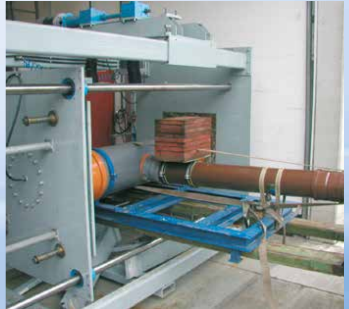
Test set-up for shear loading test
