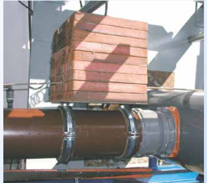
Shear loading test – 200 kg load (= 10 x the nominal diameter in N)
