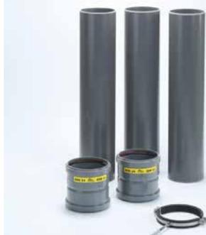
Kits in the nominal diameters of DN/OD 160 or DN/OD 200 are available for the construction of a downpipe line. Each kit consists of three pipes in the length of 750 mm, two double sockets, a stainless steel pipe clamp with a stainless steel hanger bolt and dowels.
