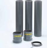
Kits in the nominal diameters of DN/OD 160 or DN/OD 200 are available for the construction of a downpipe line. Each kit consits of three pipes in the length of 750 mm, two double sockets, a stainless steel pipe clamp with a stainless steel hanger bolt and dowels.
