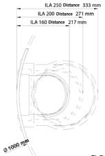
The indicated distances in the drawing are needed for the three different versions of the ILA. For the Funke-ILA 160 the distance from the chamber wall is just 217 mm, for example. This provides a non-restricted chamber accessibility.
