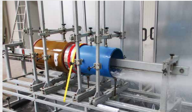
High pressure jetting test according to DIN 19523 at iro GmbH institute in Oldenburg (Germany)
