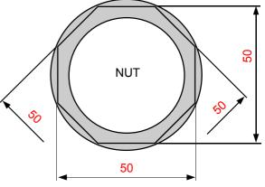
The measurement must be equal on all sides
