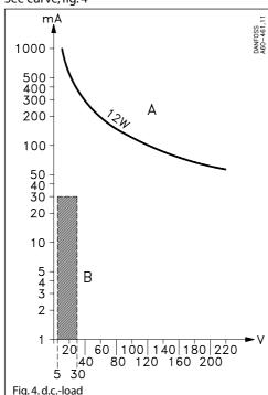
Fig. 4. d.c.-load Curve A gives the maximum load. Hatched area B: Acceptable load for the gold plating of the contact.
