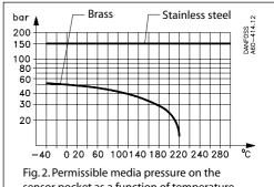
sensor pocket as a function of temperature
