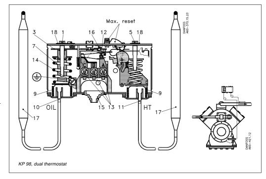
Dual thermostat KP 98 is used to provide protection against excessively high discharge gas temperature and to ensure a suitable oil temperature in the compressor.
