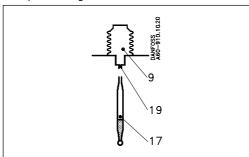
Here the interdependence between the pressure and temperature of saturated vapour is utilized, i.e. the element is charged with saturated vapour plus a small amount of liquid.
