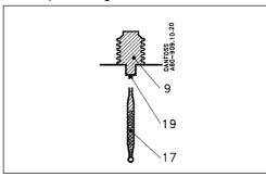
In this case the charge consists partly of a superheated gas and partly of a solid having a large adsorption surface.
