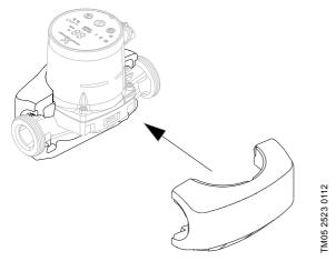
Fig. 23 Insulating shells
