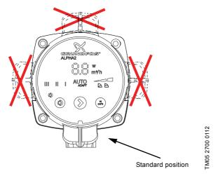
Fig. 12 Possible control box position, air-conditioning and cold-water systems
