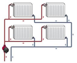
Fig. 3 Two-pipe heating system
