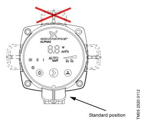
Fig. 11 Possible control box positions, heating systems
