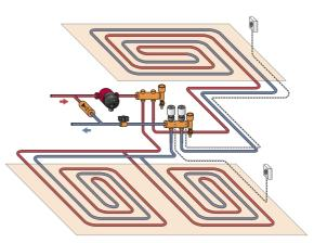
Fig. 4 Underfloor heating system
