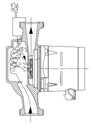
Fig. 14 Pump housing with air-separating chamber
