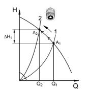
Fig. 7 Uncontrolled pump
