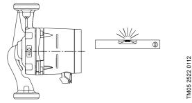
Fig. 16 Horizontal motor shaft
