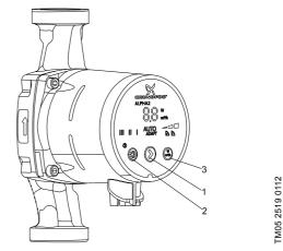
Fig. 10 Position of push-buttons
