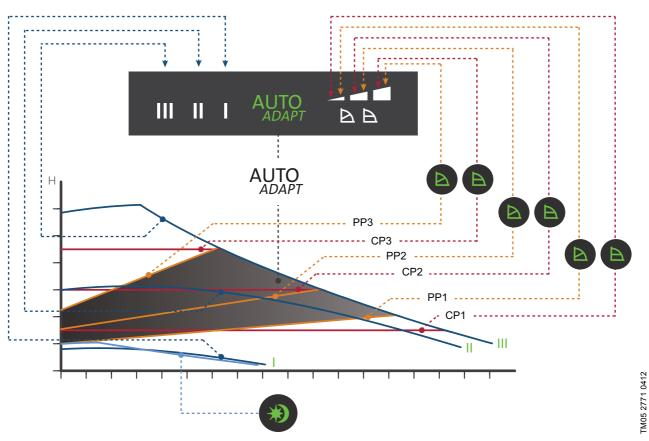
Fig. 17 Pump setting in relation to pump performance
