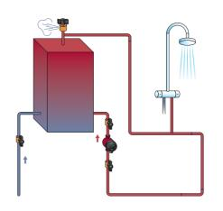
Fig. 5 Domestic hot-water recirculation system
