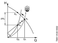
Fig. 8 Pump in proportional-pressure control mode
