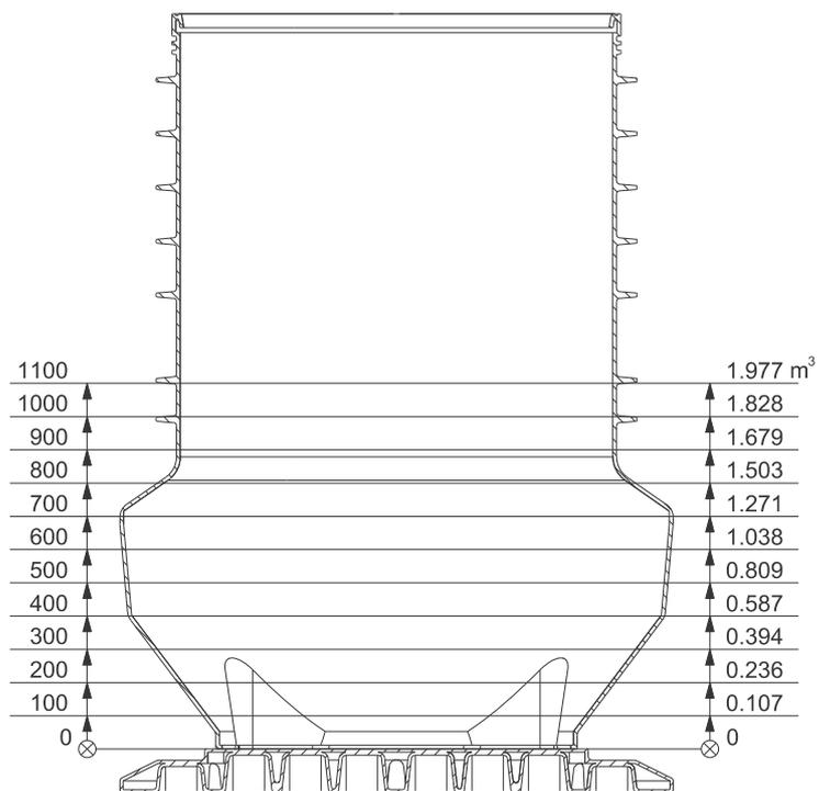
Fig. 20 Effective volume in relation to level, PUST1700
