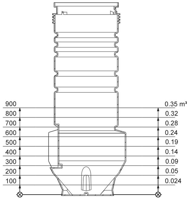
Fig. 16 Effective volume in relation to level, PUST600
