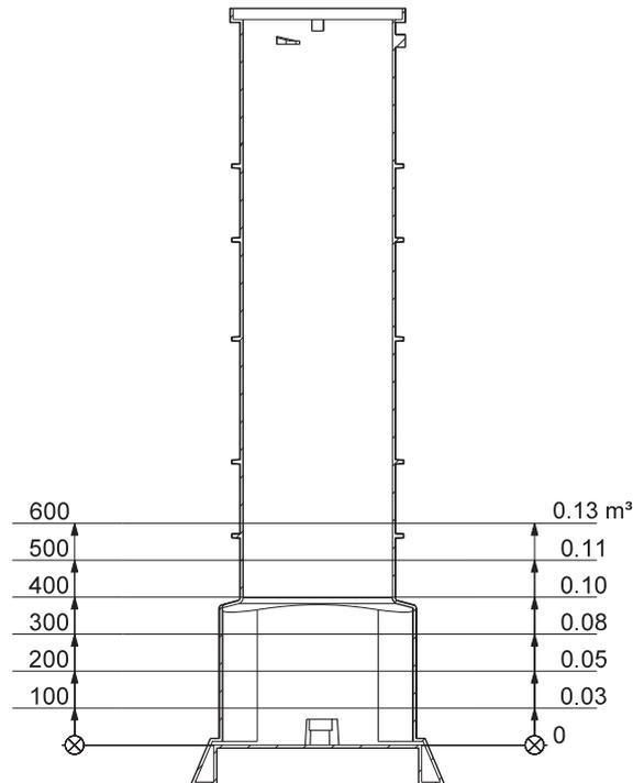
Fig. 15 Effective volume in relation to level, PUST400
