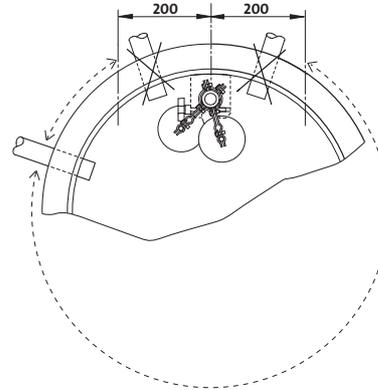
Fig. 13 Location of inlet,  $\varnothing 400\text{-}\varnothing 1000$
