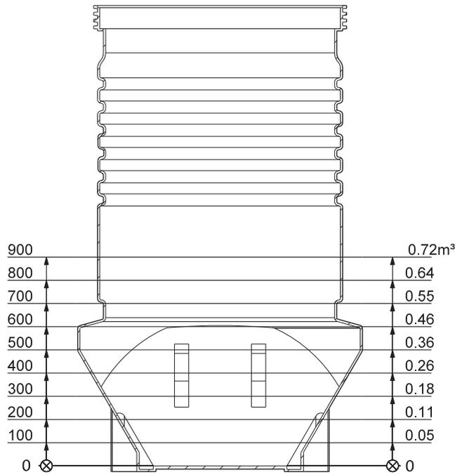
Fig. 19 Effective volume in relation to level, PUST1000 (two pumps)
