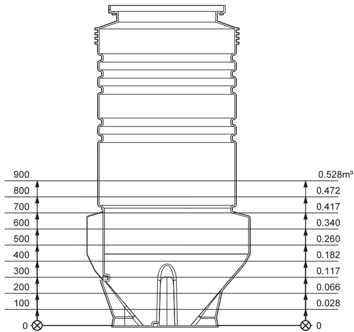
Fig. 17 Effective volume in relation to level, PUST800
