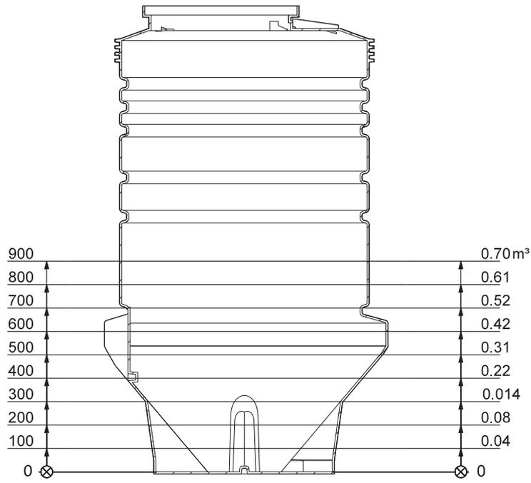
Fig. 18 Effective volume in relation to level, PUST1000 (one pump)
