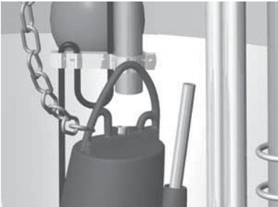
Fig. 12 Chain fitted to pump
