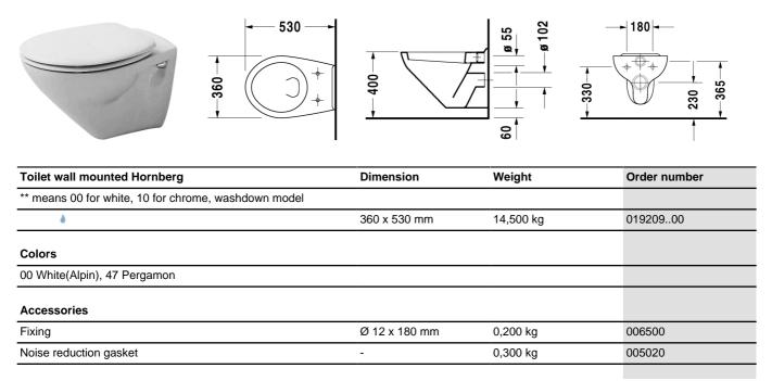
All drawings contain the necessary measurements which are subject to standard tolerances. They are stated in mm and are non-binding. Exact measurements, in particular for customised installation scenarios, can only be taken from the finished ceramic piece.
