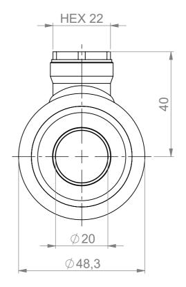
Top view of the stem without the plug
