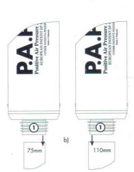
b) push-fit the rubber connector fitted to the base of the **P.A.P.A.**™ onto a 75mm or into a 110mm pipe connection.
