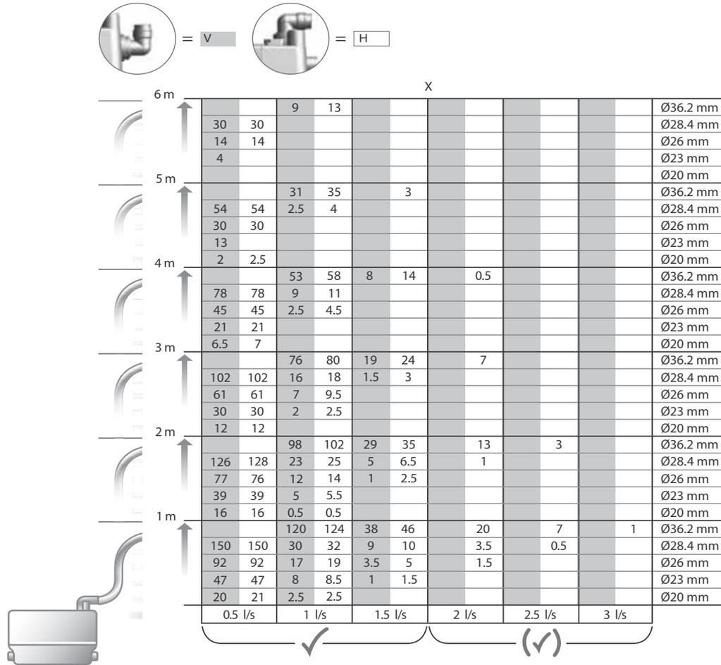
**Fig. 30** Pipe length and height in relation to inner pipe diameter and required discharge capacity
