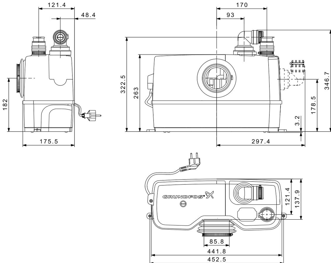
Fig. 10 Dimensional drawings, Sololift2 WC-1
