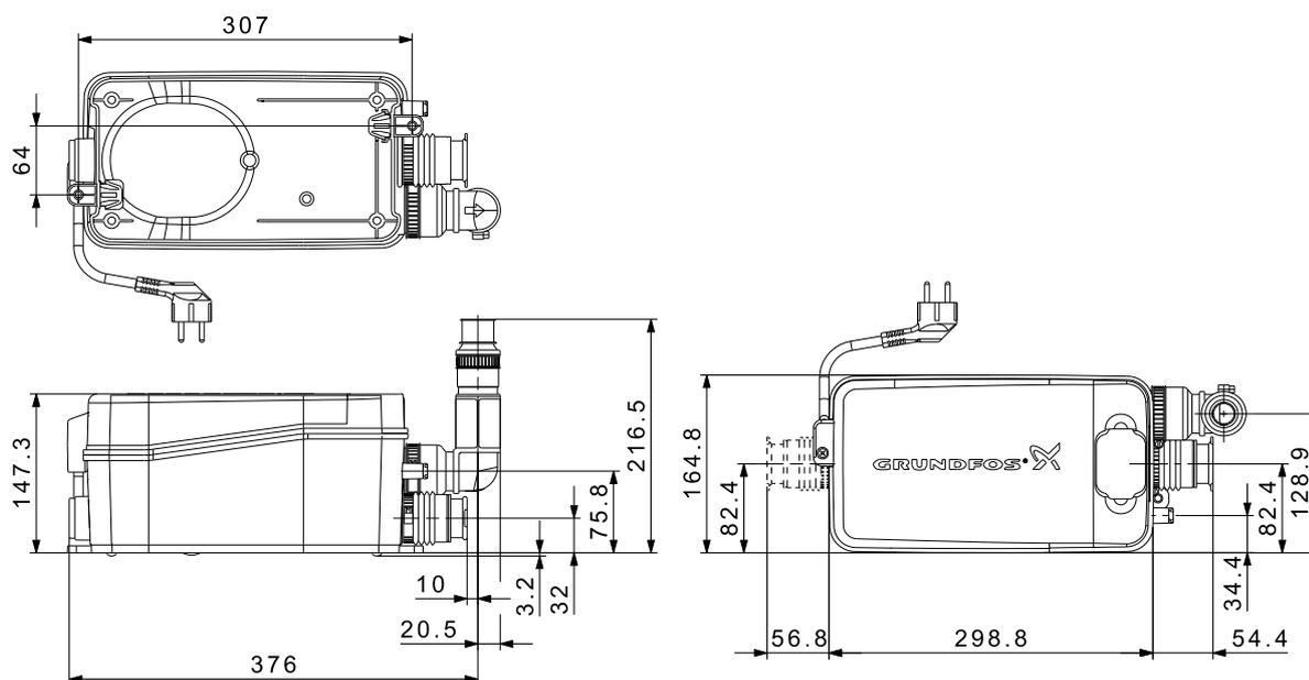
Fig. 44 Dimensional drawings, Sololift2 D-2
