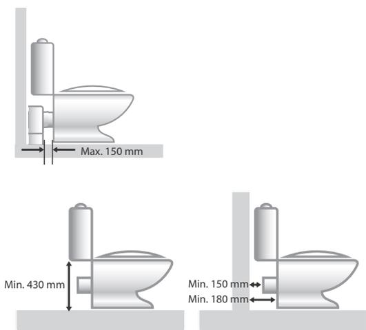
Fig. 7 Measurements to be observed
